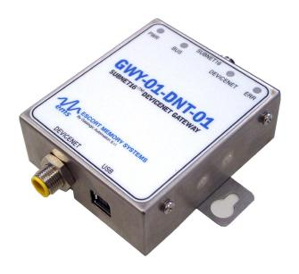
The EMS Gateway supports Subnet 16<sup>™</sup>, a subnetwork of up to sixteen EMS RFID controller/antenna stations. Subnet16 thus concentrates many read/write devices into one convenient connection point for host networks in the factory or enterprise.
